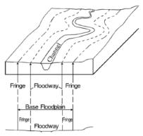
Figure 3-6: Floodway cross section and map
